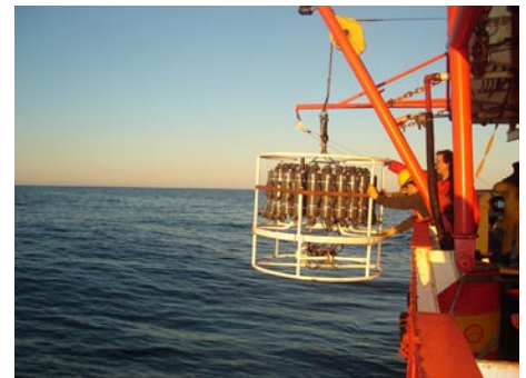
Deployment of a Conductivity-Temperature-Depth profiler in the western South Atlantic
