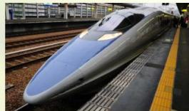
The Shinkansen Bullet Train was the fastest train in the world, traveling 200 miles per hour. The problem? Noise. Air pressure changes produced large thunder claps every time the train emerged from a tunnel, causing residents
