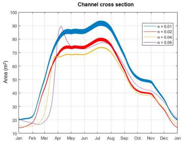
Figure 4. Sensitivity analysis of Manning coefficient ( $n$ ).
