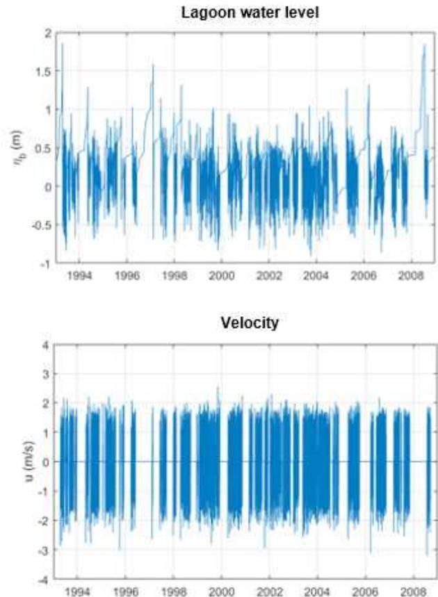
Figure 6. Water level at the lagoon and velocity at the inlet canal obtained with the physical stressor series.
