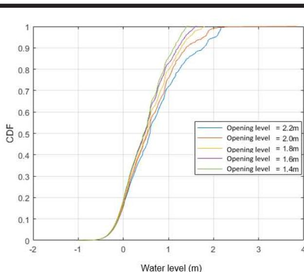
Figure 7. Empirical distribution function of the water levels obtained for the different opening values.
