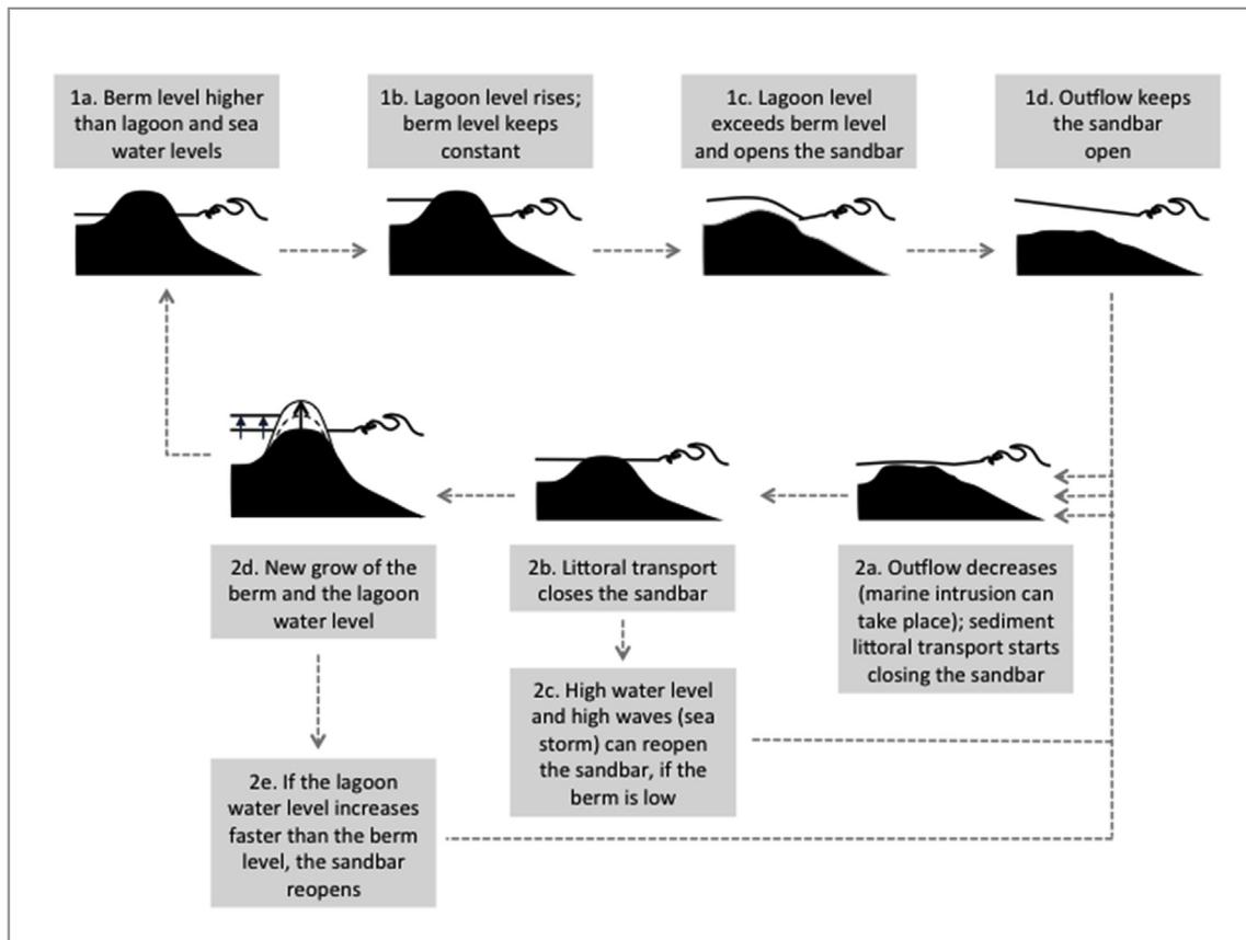
Fig. 11. Conceptual diagram of the dominant natural opening/closing mechanisms of Laguna de Rocha sand barrier (modified from Conde et al., 2015) (see text for explanation).
