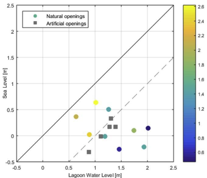
Fig. 9. Lagoon water level (LWL), sea level (SL) and significant wave height (Hs) during natural (in color) and artificial (in gray) opening events.  $SL = LWL$  and  $SL = LWL - 1$  m lines are given as reference (continuous and dashed lines, respectively). (For interpretation of the references to color in this figure legend, the reader is referred to the Web version of this article.)
