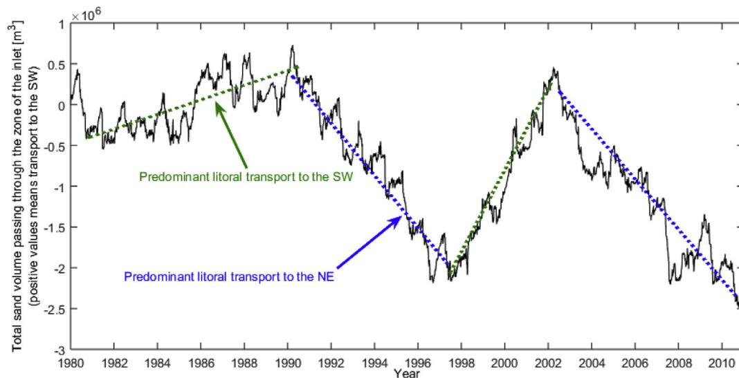
Fig. B5. Accumulated potential long-shore sediment transport through a beach profile at Laguna de Rocha inlet. Increasing values correspond to westward net transport and decreasing values correspond to eastward net transport.
