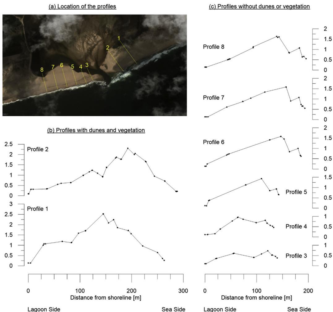
Fig. 8. Profiles of the sand barrier. (a) Location of the profiles; (b) Profiles with dunes and vegetation, located outside of the area where the lagoon usually opens; (c) Profiles without dunes or vegetation, located in the area where the lagoon usually opens.
