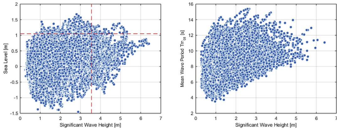
Fig. B2. Scatter plots of significant wave height ( $H_s$ ) and sea level (left) and significant wave height ( $H_s$ ) and mean wave period (right).
