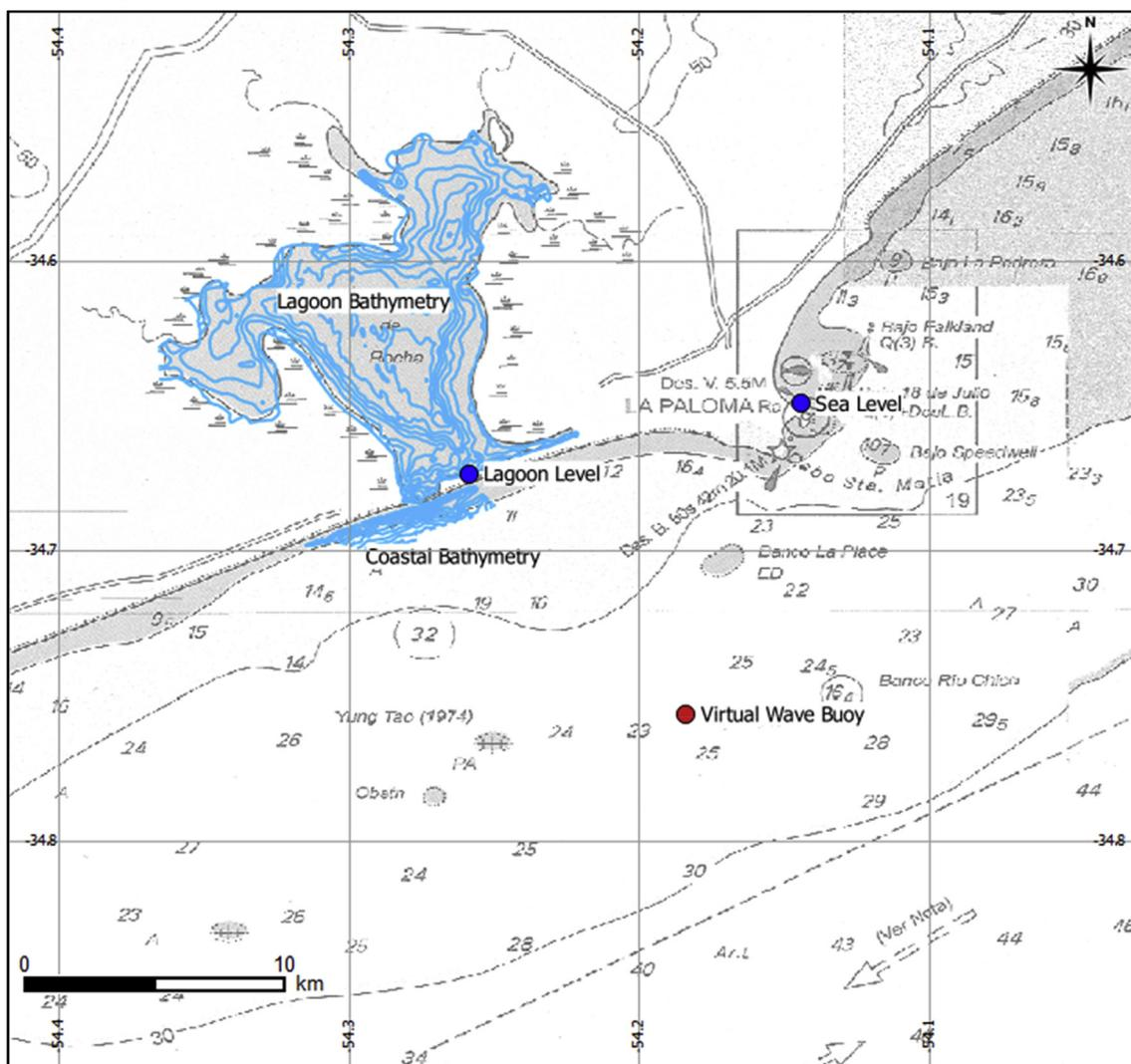
**Fig. B1.** Bathymetry from the nautical chart (in gray scale), Laguna de Rocha and nearshore area surveyed bathymetry (light blue), location of lagoon water level and sea level gauges (blue dots) and location of the wave virtual buoy (red dot).
