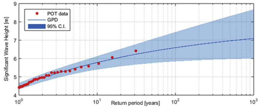
Fig. B3. Extreme value probability distribution of wave height ( $H_s$ ) at the virtual buoy: data (dots) and generalized Pareto distribution (line) fitted to the data, along with the 95% confidence interval.
