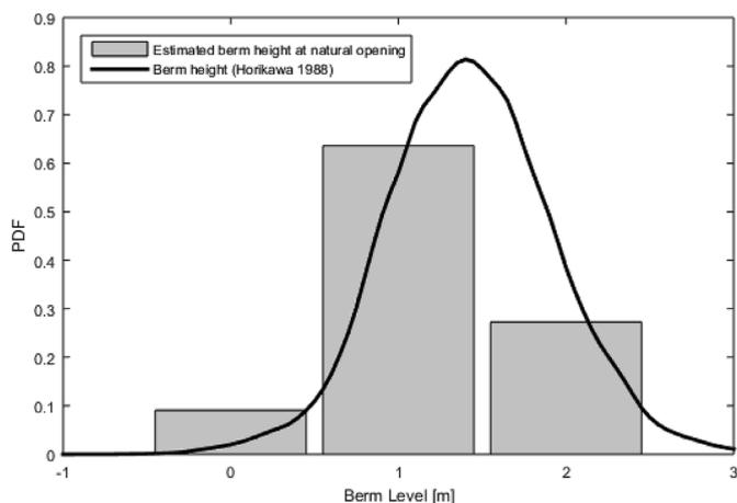
Fig. 10. Probability density function (PDF) of berm heights calculated with equation (2) (continuous lines) and frequency of berm heights estimated assuming berm heights equal to lagoon water levels during natural openings (bars).
