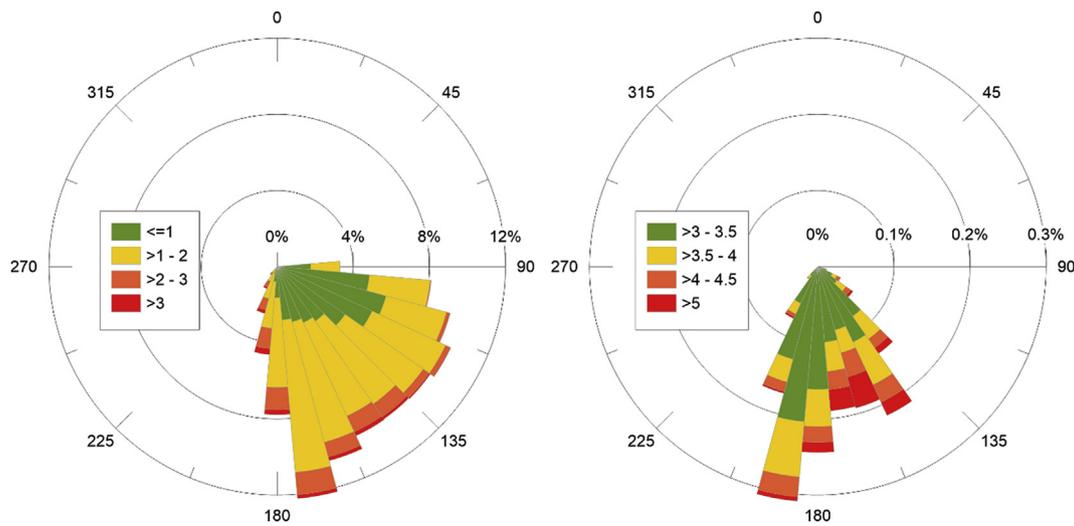
Fig. B4. Wave roses at the virtual buoy (see Fig. 2). Left: all data. Right: data with wave height ( $H_s$ ) > 3 m. Colors refer to significant  $H_s$ .
