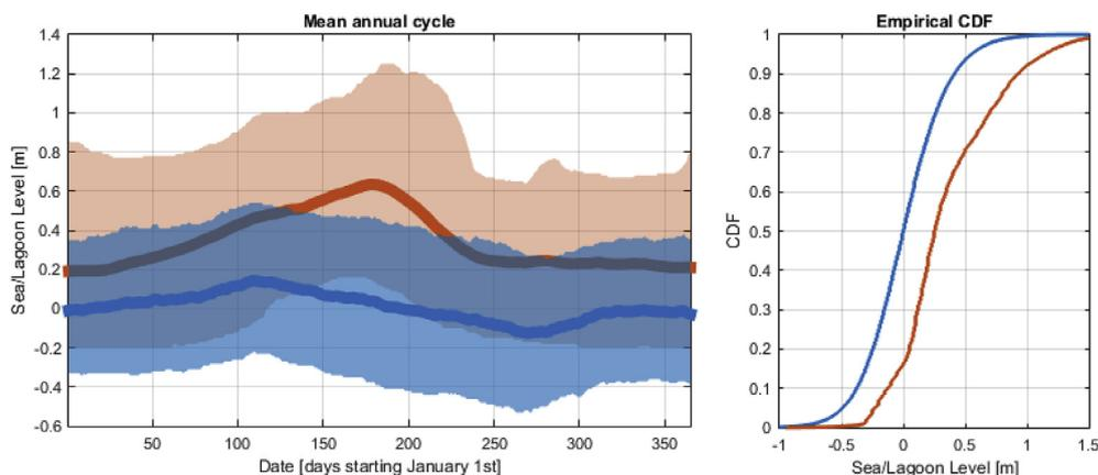
**Fig. 6.** Analysis of the lagoon water level (red) and sea level gauges at La Paloma harbor (blue). Left: mean annual cycles (mean value and range 10%–90% quantiles). Right: empirical cumulative distribution functions. (For interpretation of the references to color in this figure legend, the reader is referred to the Web version of this article.)
