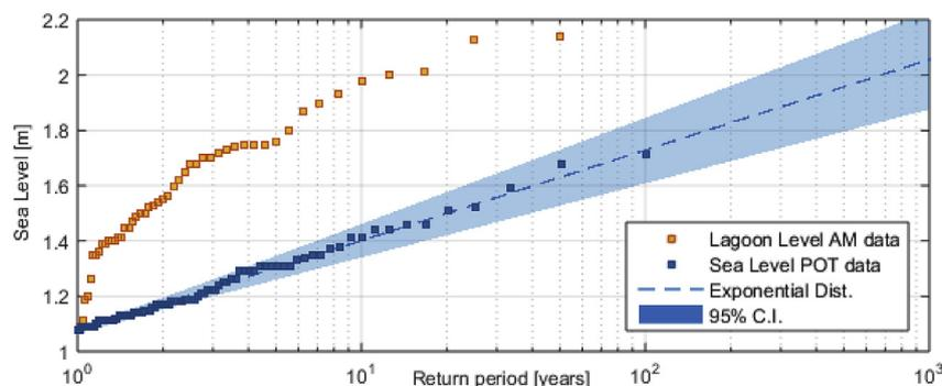
**Fig. 7.** Extreme value analysis of the lagoon water levels (red) and of sea level gauges at La Paloma harbor (blue). (For interpretation of the references to color in this figure legend, the reader is referred to the Web version of this article.)
