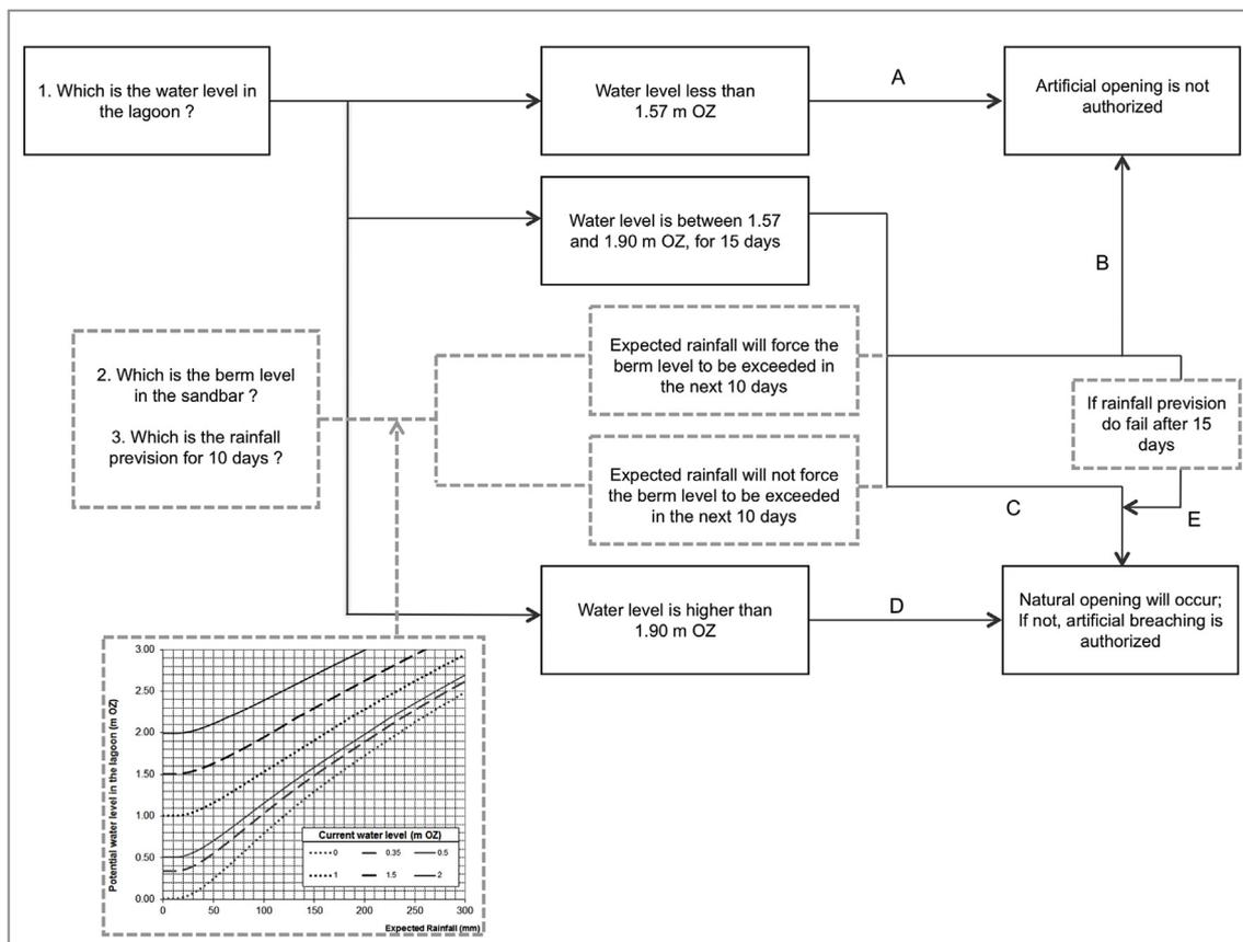
Fig. 12. Decision-making model for the artificial opening of Laguna de Rocha sand barrier (modified from Conde et al., 2015). Questions 2 and 3 arise in the protocol 5 days after water level enters the 1.57–1.90 m OZ range. Inset left below is a chart for the estimation of the probable water level of Laguna de Rocha, derived from the actual water level and the rainfall prediction.
