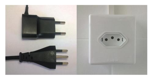
The outlet works on plugs with either two or three pins (the third pin is the optional 'earth' pin), but the plug must have this shape. We recommend getting an international power plug adapter and avoid any problems of running out of batteries.
