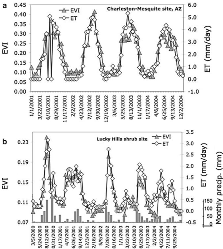
**Fig. 26.6** MODIS EVI-eddy covariance tower ET relationships at riparian (a) and upland shrub (b) vegetation communities at the SMEX04 site in southeast Arizona, using MOD13Q1. The strong evaporation component in the upland shrub site during rain events results in significant departures from seasonal EVI values (tower flux data provided by Bill Emmerich and Russell Scott, USDA-ARS Southwest Watershed Research Center, Tucson, AZ)
