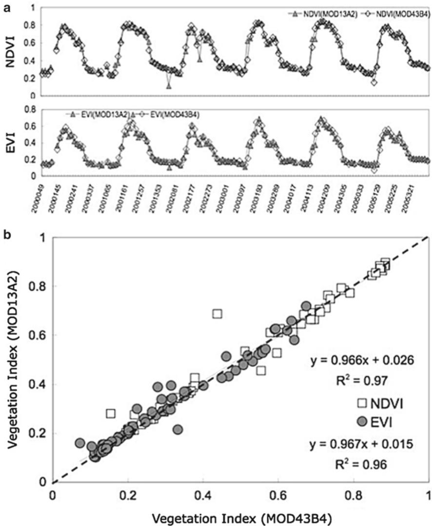
**Fig. 26.4** Comparison of MODIS 1-km VI (MOD13A2) with 1-km NBAR generated VI (MOD43B4) for the Konza Prairie site, Kansas, United States over 6 years (a); and linear regression of MOD13A2 with MOD43B4 VIs for Konza Prairie, Lucky Hills shrub site in Arizona, and Harvard Forest in Massachusetts (b)
