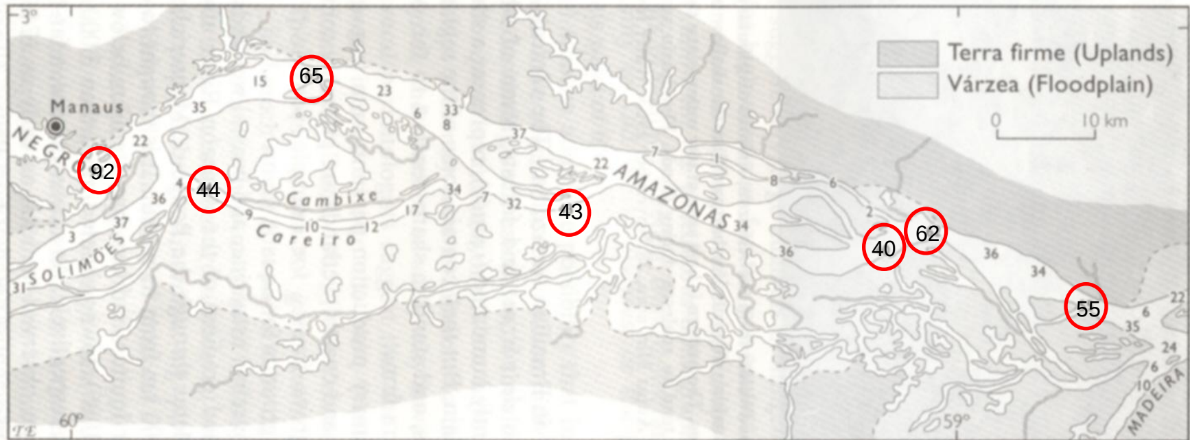
Figure 6.4 Stretch of the Amazon River, showing lenticular islands dividing the stream-bed into a master channel and one or more side channels, or paranás . Selected soundings (in metres) from the 1967 hydrographic survey by the Brazilian Navy; datum is mean lower low-water stage. (Taken, together with most water surface lines, from Brasil, Rio Amazonas, Cartas de Praticagem da Flotilha do Amazonas , Marinha do Brasil, Sheets P 4 106 A and B, 2nd ed., 1970. Original scale 1:100,000. Approximate outline of terra firme lakes, and boundary between uplands and floodplains, from aerial photographs.)
