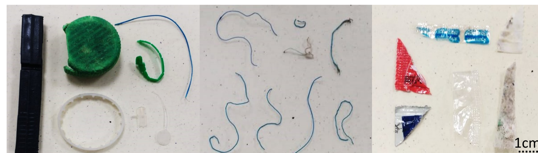
Figure 3. Material collected in Moçambique beach, Ribeirão da Ilha beach and Lagoinha do Norte beach, containing plastic tags (seal tag), seals, cloth peg, bottle caps, fibers, straw, toothpick packing material and sachets.
